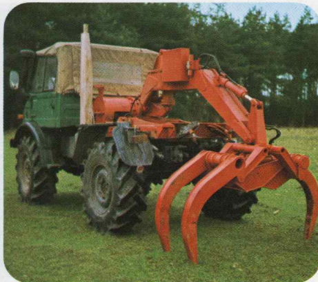
In the process of extracting and thinning, very large loads of timber can be carried by means of a log skidder operated by one man.
