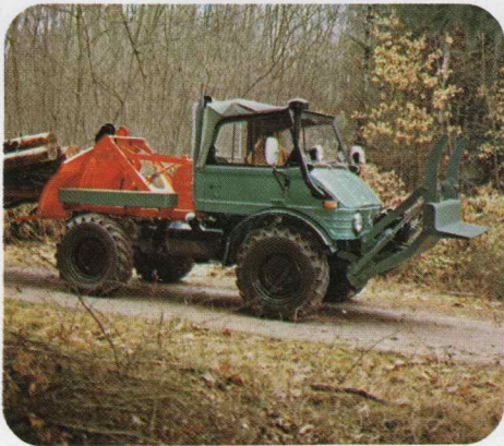
Special light-timber carrying equipment with raised fairleads and large rear plate for U 600.
