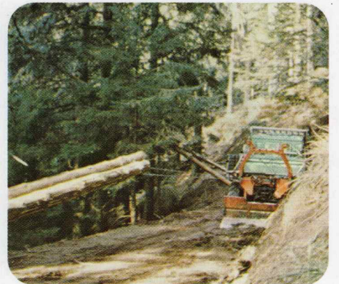
The Unimog forestry tractor with double drum winch and sprag works very efficiently when hauling timber on steep slopes.
