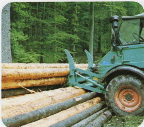
The front-mounted stacking unit is a perfect addition to the logging equipment. It speeds up, simplifies and facilitates operation.
