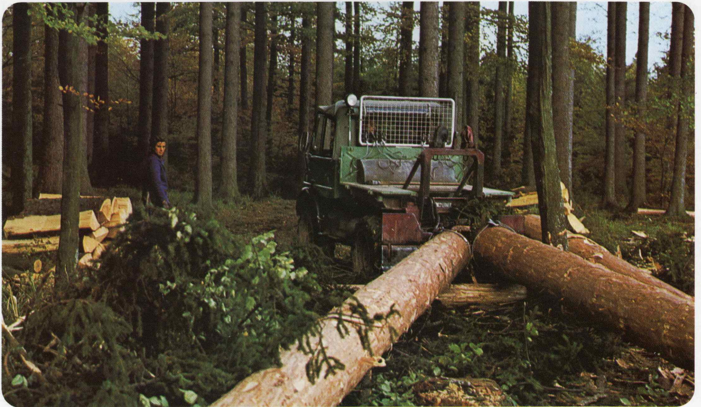
Excellent manoeuvrability on difficult terrain and high ground clearance – well-known features of the Unimog forestry tractor – often allow direct skidding of timber.
