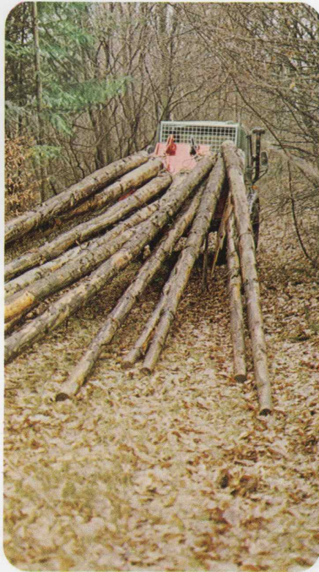
The large and sturdy rear protection plate of the U 600 permits the moving of large bundles of light timber.
