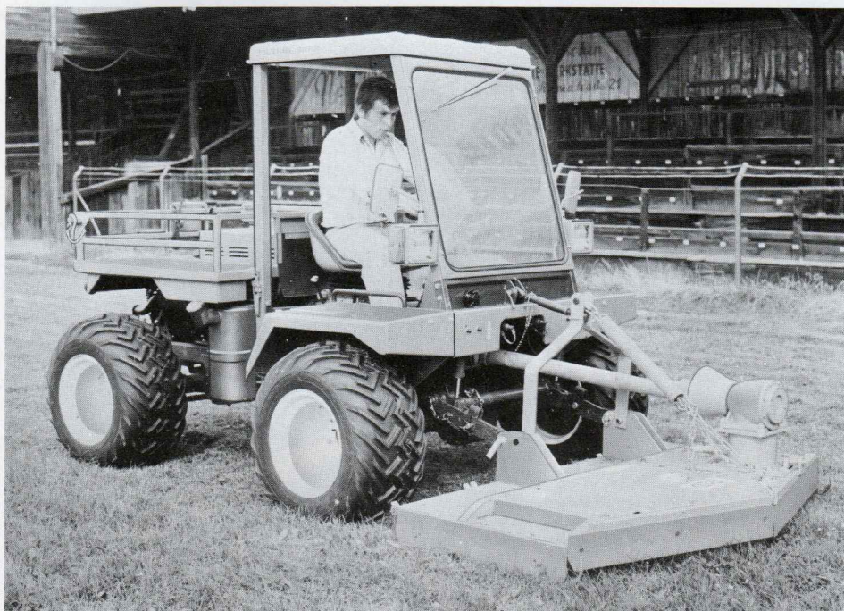
Rotary Lawn Cutter VOTEX A3 1801, working width 1,80 m, 3 straight knives driven off the front-pto via a V-belt. Robust,
