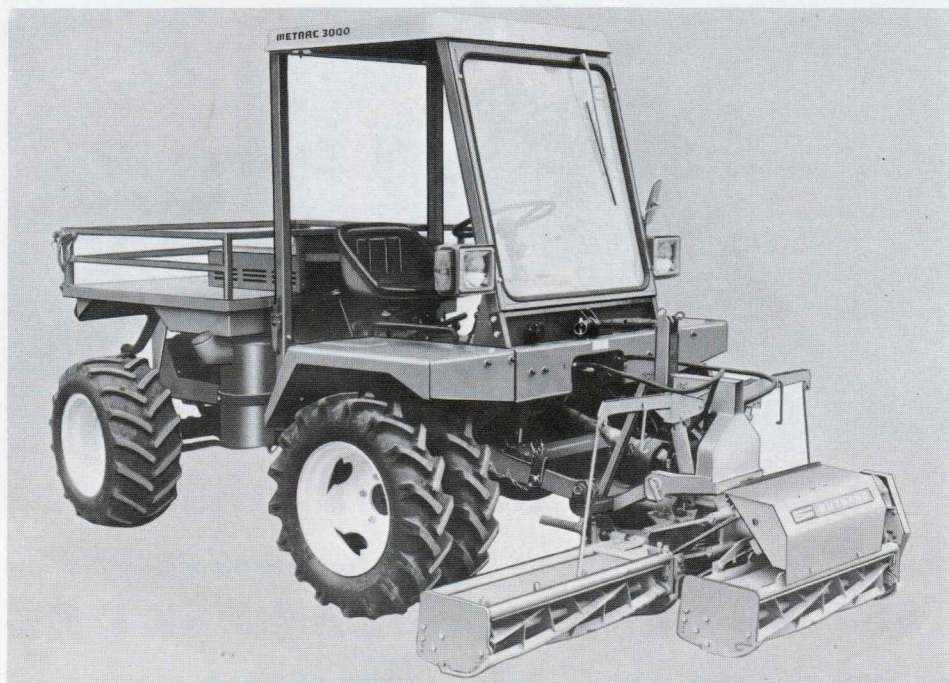
Three-Cylinder type Lawn Cutter, working width 2,30 m, driven by front pto. For
