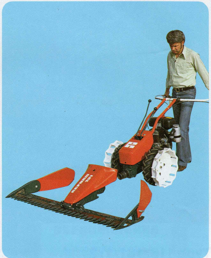
wear-resistant oilbath-mower drive with new, easy-to-maintain knife head
