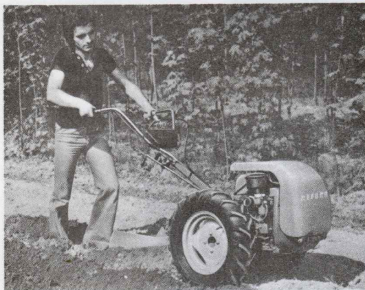
Ridge plough adjustable with 5,00—12 tyres for hilling-up and furrowing.
