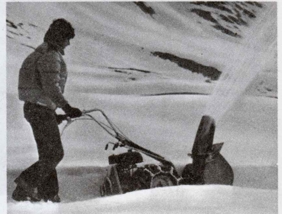
Rotary snow-plough 60 cm working width with rotatable ejection funnel.
