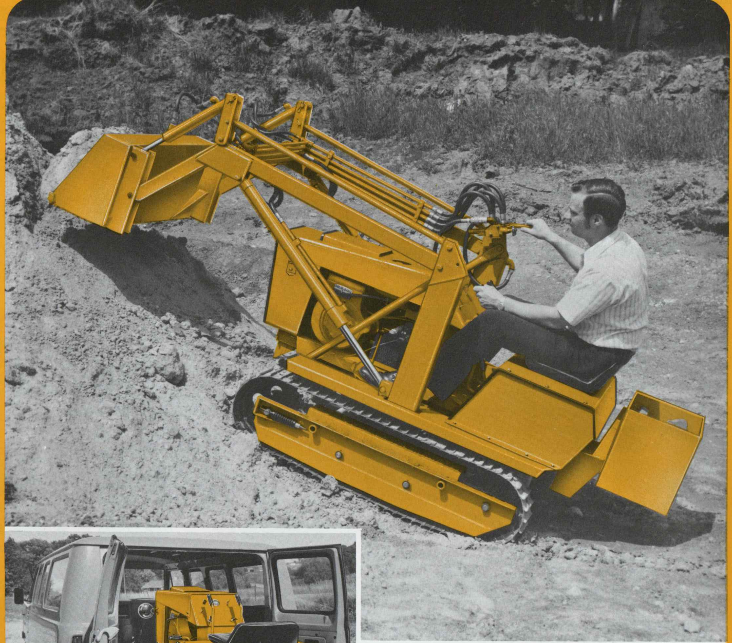
This front-mounted high lift loader with hydraulic lift can be attached in minutes without special tools. A low lift loader with electric lift system is also available. (Inset) Its 41" width makes Magnatrac easier to transport by truck to distant work sites.
