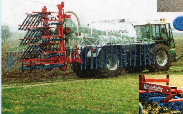
SPRING TINE HARROW, 4,5 M WIDTH, IN WORKING POSITION, BEING TOWED
