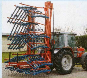
SPRING TINE HARROW, 15 M WIDTH, IN TRANSPORT POSITION
