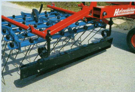
SPRUNG LEVELLER BAR 1,5 M TO LEVEL COWDUNG AND MOLE-HILLS.
