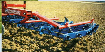
SPRING TINE HARROW, 4,5 M WIDTH, IN WORKING POSITION, BEING TOWED
