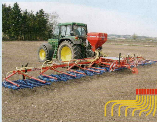
SPRING TINE HARROW 6M WITH PNEUMATIC SEEDER AIR 8, RNOVATING PASTURES
