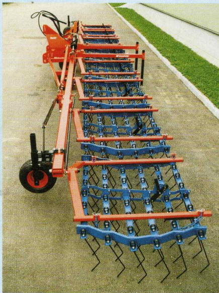
SPRING TINE HARROW, 12 M WIDTH, IN WORKING POSITION, TRANSPORT WIDTH LESS THAN 3M
