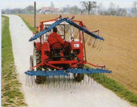
SPRING TINE HARROW, 6 M WIDTH, TRANSPORT SETTING, 2,80 M TRANSPORT WIDTH
