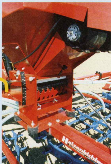
PNEUMATIC SEEDER AIR 8, WITH TRANSMISSION INFINITELY VAIABLE, SEED METERING ROLLER AND 2 ELECTRICALLY DRIVEN FANS. FOR FITTING ON EXISTING HARROWS - SOWING AND OVERSOWING
