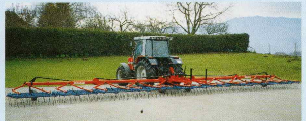
SPRING TINE HARROW, 15 M WIDTH, IN WORKING POSITION
