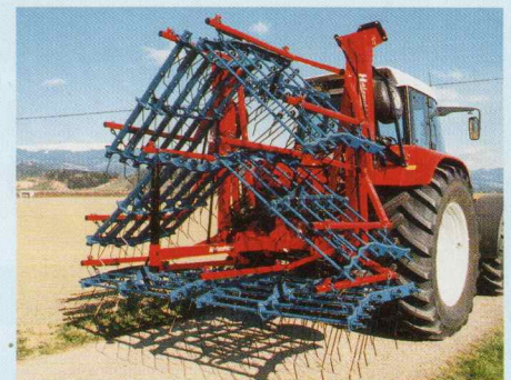
SPRING TINE HARROW, 9 M WIDTH, (TRANSPORT POSITION)
