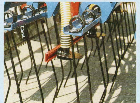
(OVERSOWING) DEFLECTORS MOUNTED ON HARROW SECTION
