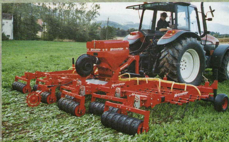
AIR 16, fitted on 6 m Vertikator, for sowing and oversowing
