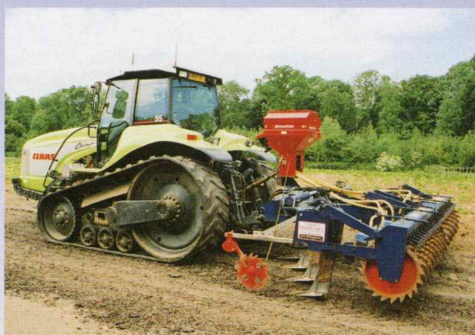
AIR 8 fitted on a sub-soiler, to broadcast green covers
