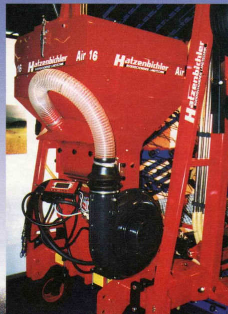
Air 16, fitted on comb harrow 12 m (position transport)
