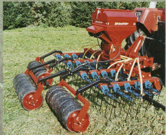
AIR 8 fitted on 3 m Vertikator for the regeneration of the grassland, for sowing and oversowing
