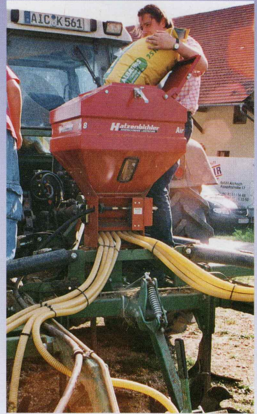
AIR 8 during refilling of the tank (big lid for easy refilling, big window to control seed level)
