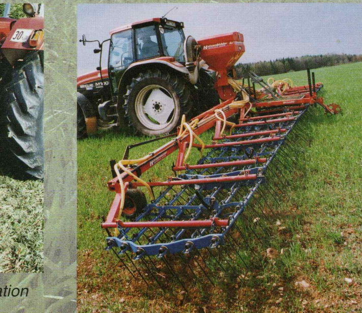
AIR 16, fitted on comb harrow 12 m (sowing grass, clover into cereals)
