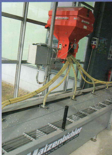
On the test unit of the Hatzenbichler Company, different seeds are being tested for their broadcast abilities
