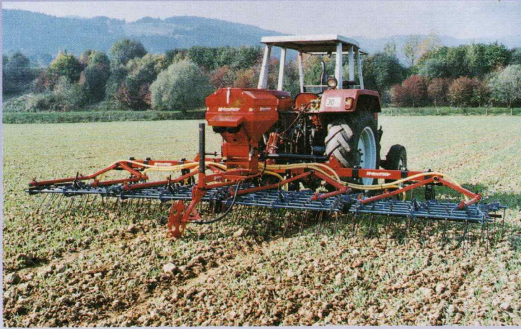
AIR 8, fitted on comb harrow 6 m (sowing grass-clover mixtures into cereals)
