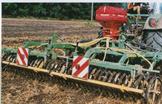
AIR 8, fitted on a chisel plough, foldable, to broadcast green covers
