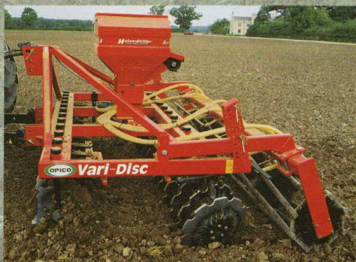
AIR 8, fitted on a disc harrow, to broadcast green covers or for sowing
