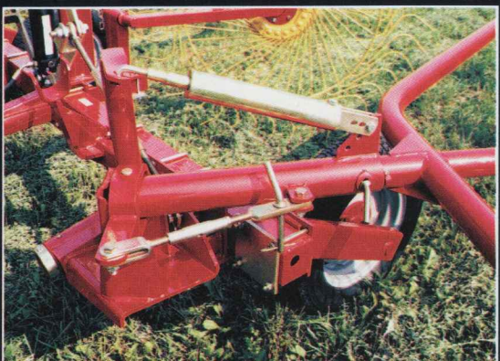
Shock absorbing floating spring and adjusting turnbuckle
