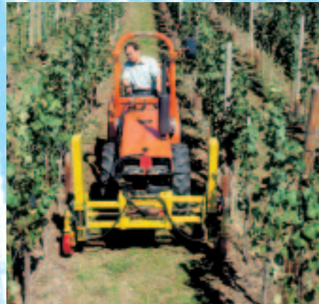
a front mounted unit optimizes the mechanical treatment under the vines
