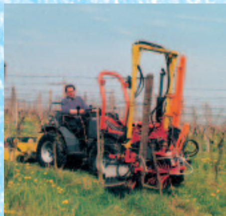
rotating brooms enable an economical and environmentally friendly method of clearing between the vines
