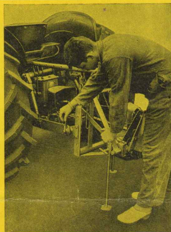
Mounting the mower frame to the tractor drawbar. The mower is conveniently positioned on its two supporting legs.
