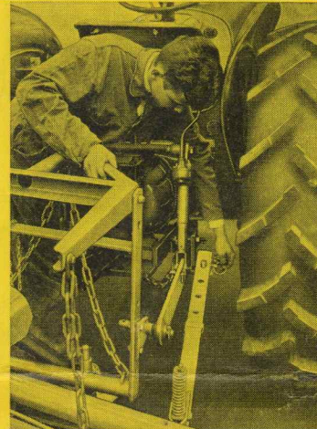
The power transmission shaft is provided with swift hitch device and is easily mounted to the tractor's p.t.o. shaft, without tools.
