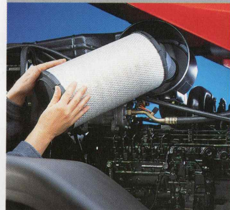
The dual element filter is easily checked.
