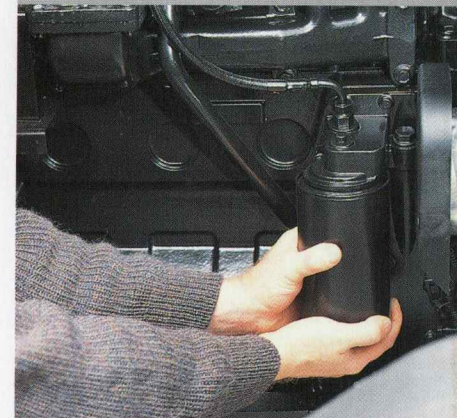
The dual element filter is easily checked.
