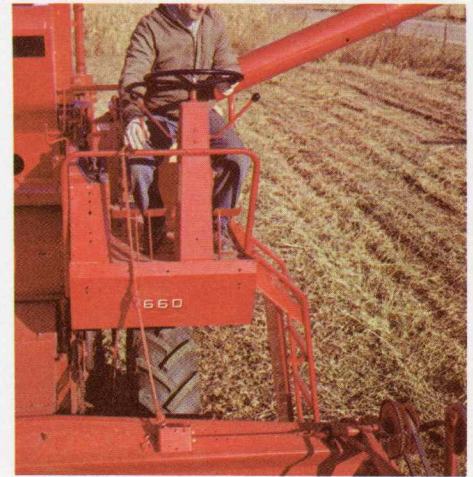
Remote control of reel speed attachment lets you match reel or pickup speed to conditions precisely from the driver's seat.
