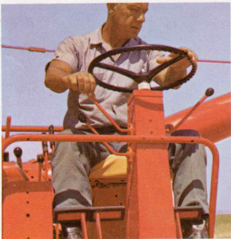
Hydraulic header control. This lever adjusts header height from 2 \frac{3}{8} inches below to 32 \frac{1}{2} inches above ground level.
