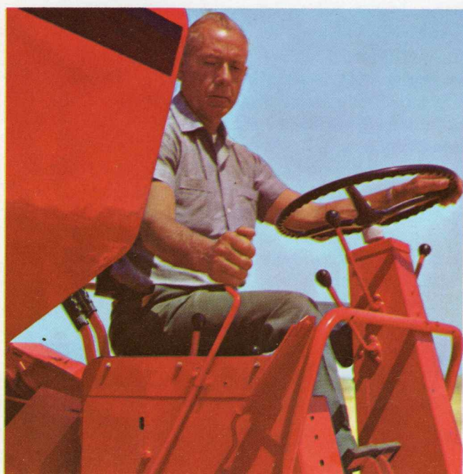
Adjusting concave clearance. Gauge shows the exact clearance.
