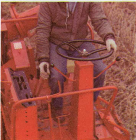
Header throughput lever stops or starts cutting-feeding mechanism . . . helps stop foreign objects, helps feed bunched windrows evenly.
