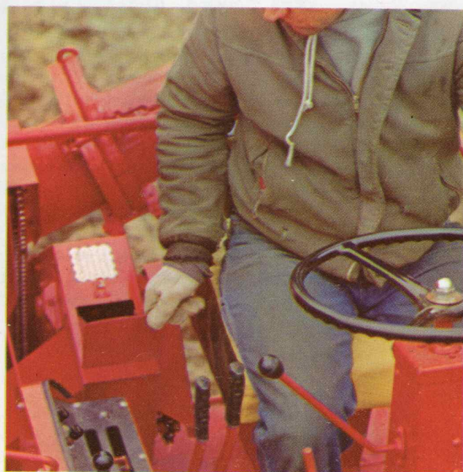
Checking tailings. Just flip up the door at your right elbow.
