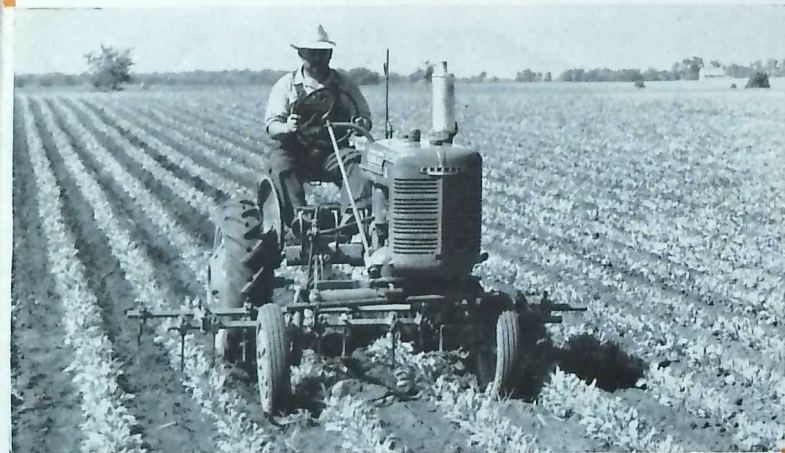
Farmall-A and the A-435 vegetable cultivator. This is the cultivator for beets, beans, lettuce, carrots, onions, etc. A wide range of combinations is available for cultivating flat or bedded plantings. Rows can be spaced as closely as 12 inches apart.
