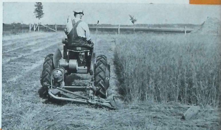
Farmall-A and this simple, practical No. 16-A mower will cut 20 or more acres a day. The sickle is belt-driven. The power take-off attachment supplies the power. A safety device prevents breakage should the cutter bar strike an obstruction.
