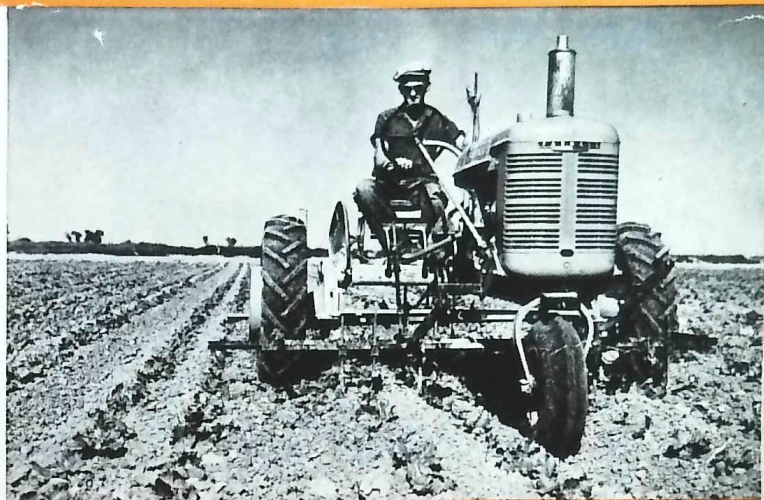
Farmall-B and the B-435 vegetable cultivator. This is the cultivator for beets, beans, lettuce, carrots, onions, etc. A wide range of combinations is available for cultivating flat or bedded plantings. Rows can be spaced as close as 12 inches apart.
