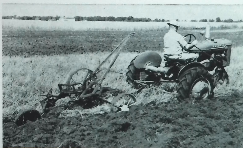
Farmall-B and the No. 3 Little Wonder plow. Farmall-B will pull this plow with a 16-inch bottom in third speed under average conditions—4 \frac{3}{4} miles an hour—6 or 7 acres a day.
