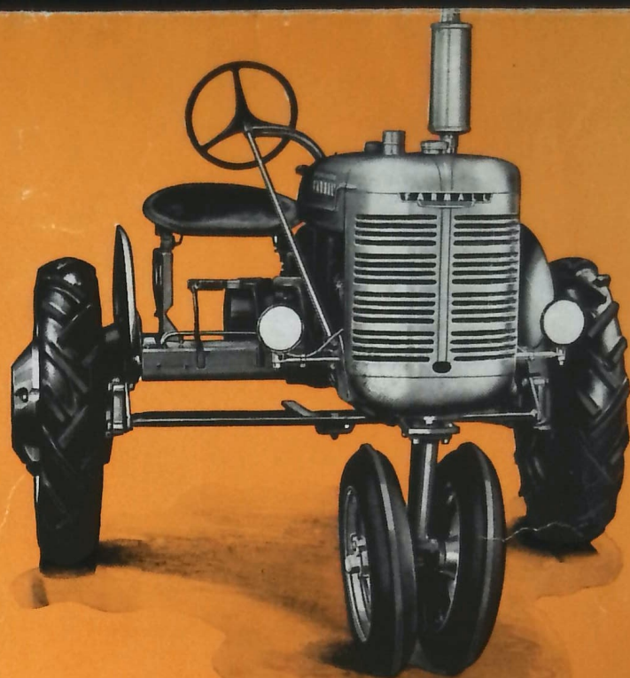
A front view of the Farmall-B, showing the offset seat. The operator sits comfortably and looks straight ahead at his work. The tractor is here shown with double front wheel, belt pulley, lighting, and muffler attachments, and rear wheel weights.
