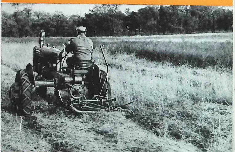
The Farmall-B tractor equipped with the No. 16-B mower will cut up to 4 acres an hour. The outfit can be operated all day long on 6 to 8 gallons of fuel.
