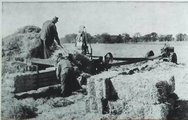
The Farmall-B is shown here operating the No. 15 hay baler. Its economy in all hayfield operations makes this little tractor a splendid auxiliary machine on the larger farms.
