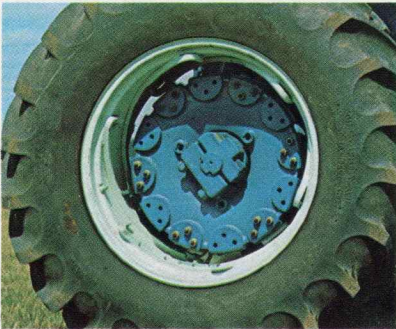
Optional power-adjustable wheels (with 16.9 inch tires) adjust through the full 60" to 97" (152 to 246 cm) tread range, without reversing the rims.
