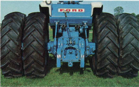
Dual wheel option is available for 34" and 38" (86 cm and 96 cm) diameter power-adjustable wheels.
