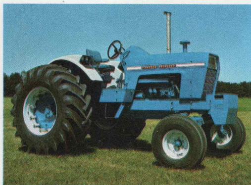
Wide front axle, set up for 108" (275 cm) wheelbase.
