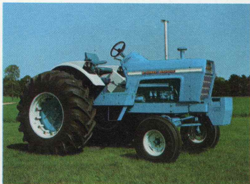
Axle set up for 91.5" (232 cm) wheelbase.
