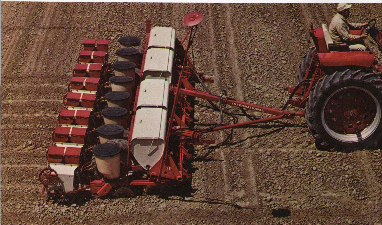
58 Series 8-row plants 30-inch rows. Available with either 2,000 pounds capacity metal fertilizer units or 2,200 pounds fiberglass fertilizer units.
