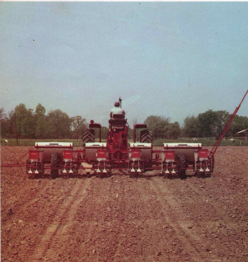
56 Series 6-row plants 36 or 38" rows and is available with either 1,500 pound capacity metal or 1,650 pound capacity fiberglass fertilizer hoppers, also with three 50 gallon liquid fertilizer tanks.
