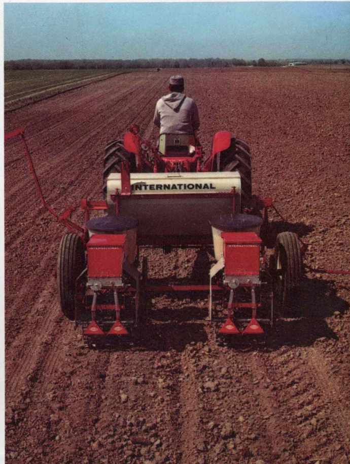
56 Series 2-row plants 28 to 40-inch rows. Available with 500 pound metal fertilizer unit or with 50 gallon liquid fertilizer tank.
