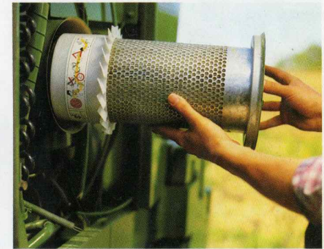
Air filter automatically discharges dirt through a special valve, extending service intervals. Easy access and simplified daily servicing encourage regular maintenance.
