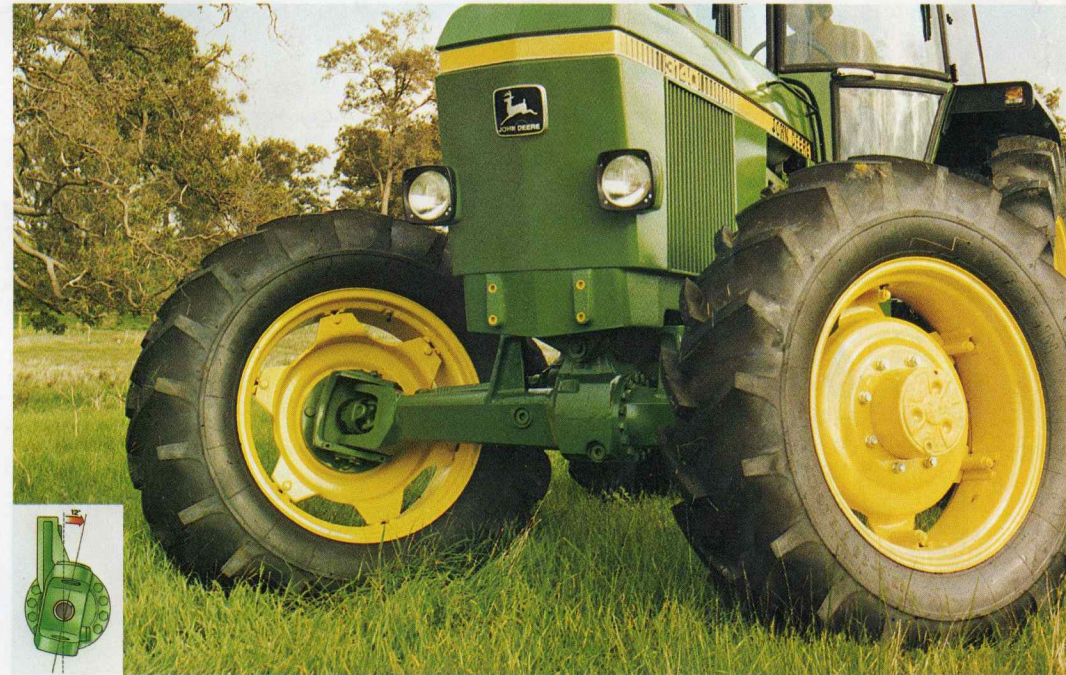
Exclusive 12-degree castor angle (inset) allows front wheels to lean, when turning, to give a tight turning circle. Centre driveline and slim axle give excellent ground clearance.
