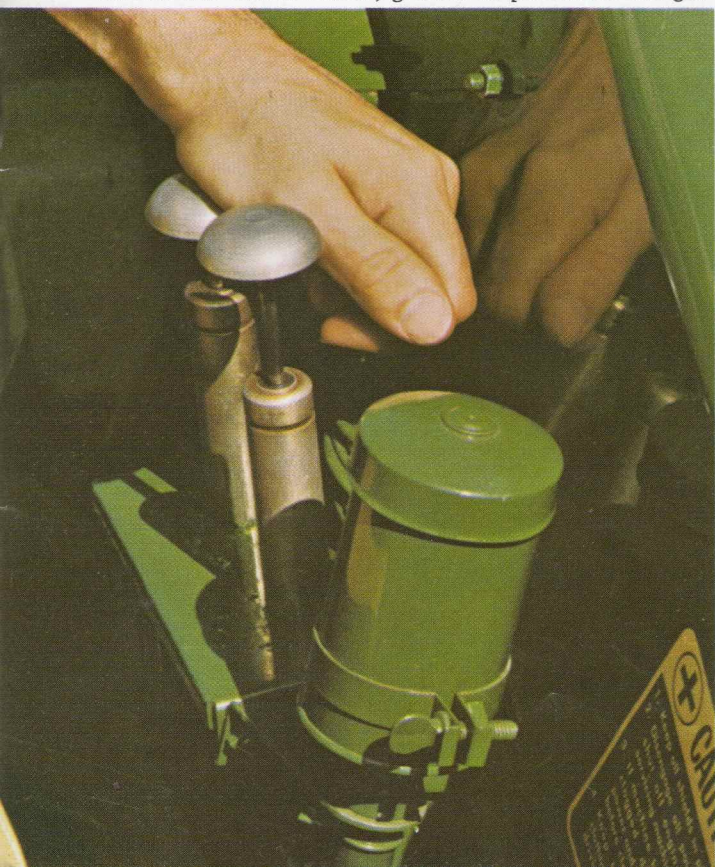
Stroke the Multi-Luber, grease 48 points on-the-go.
