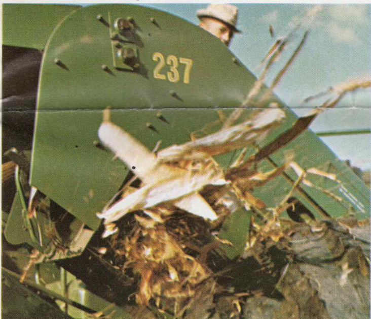
Husk clean with serrated rubber against steel spirals.
