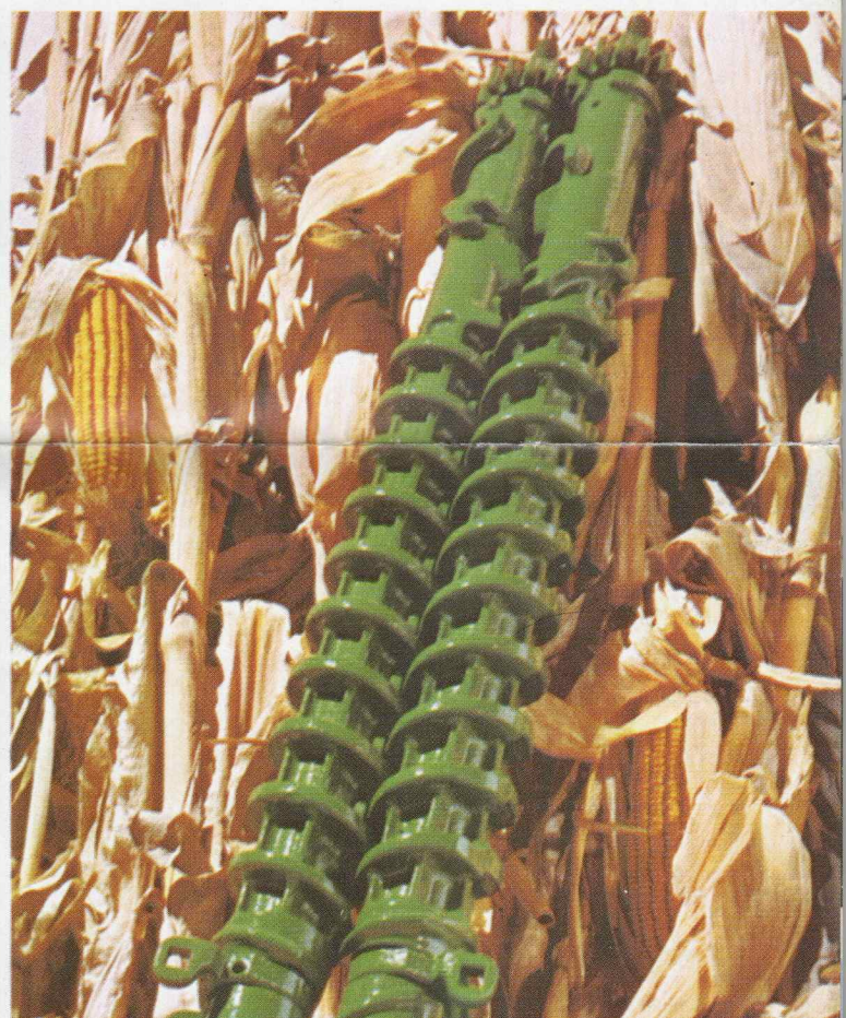
Down stalks seldom escape three gathering chains.
