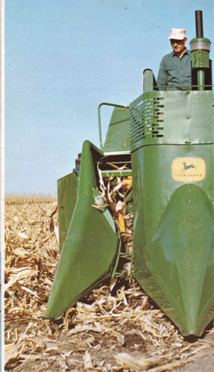
Tall inside and outside shields save high ears.
