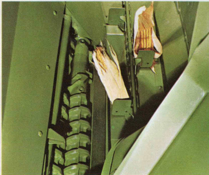
Husks are augered out behind the rear tractor tire.
