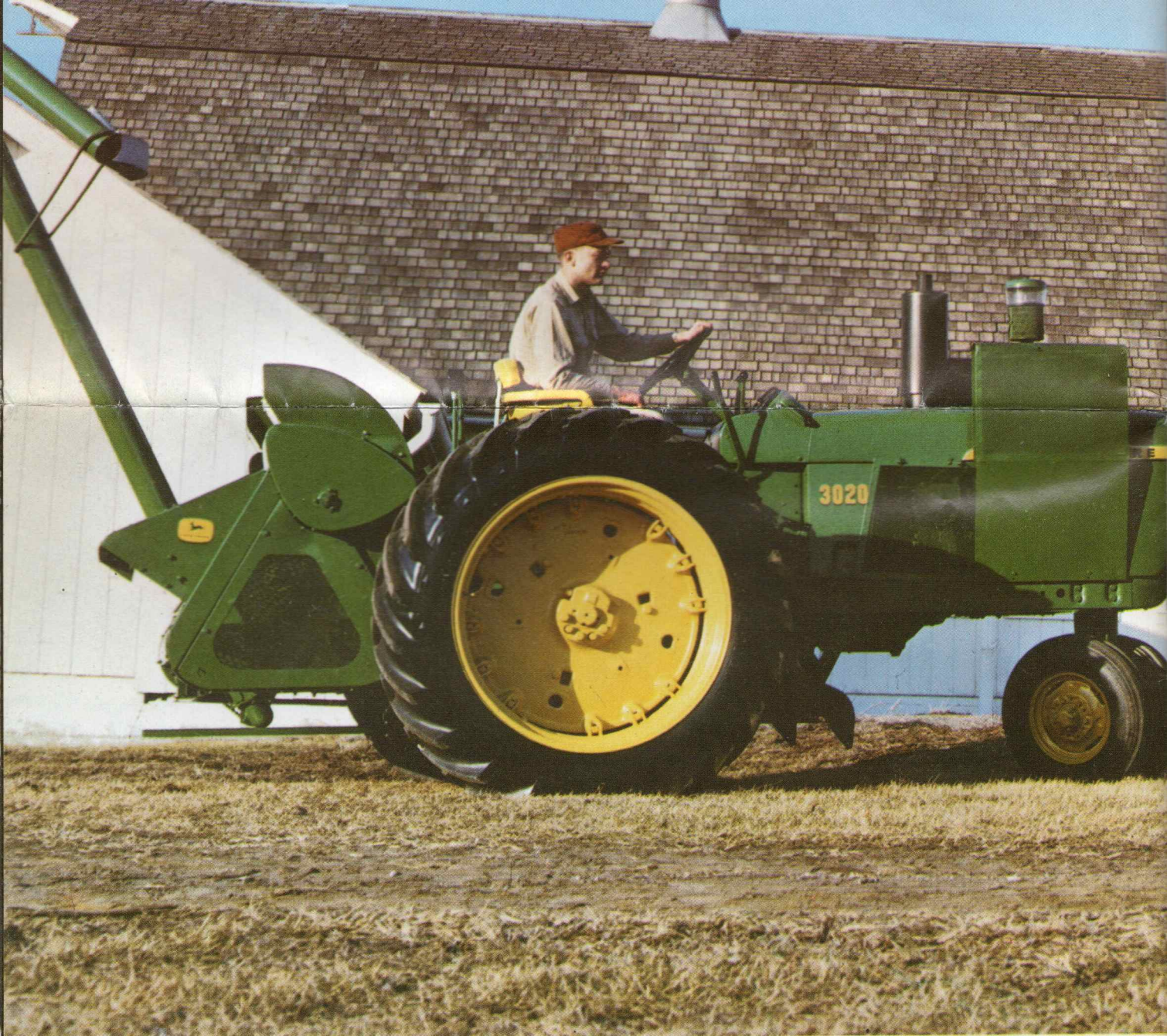
Move this lever to start wagon elevator after a turn.
