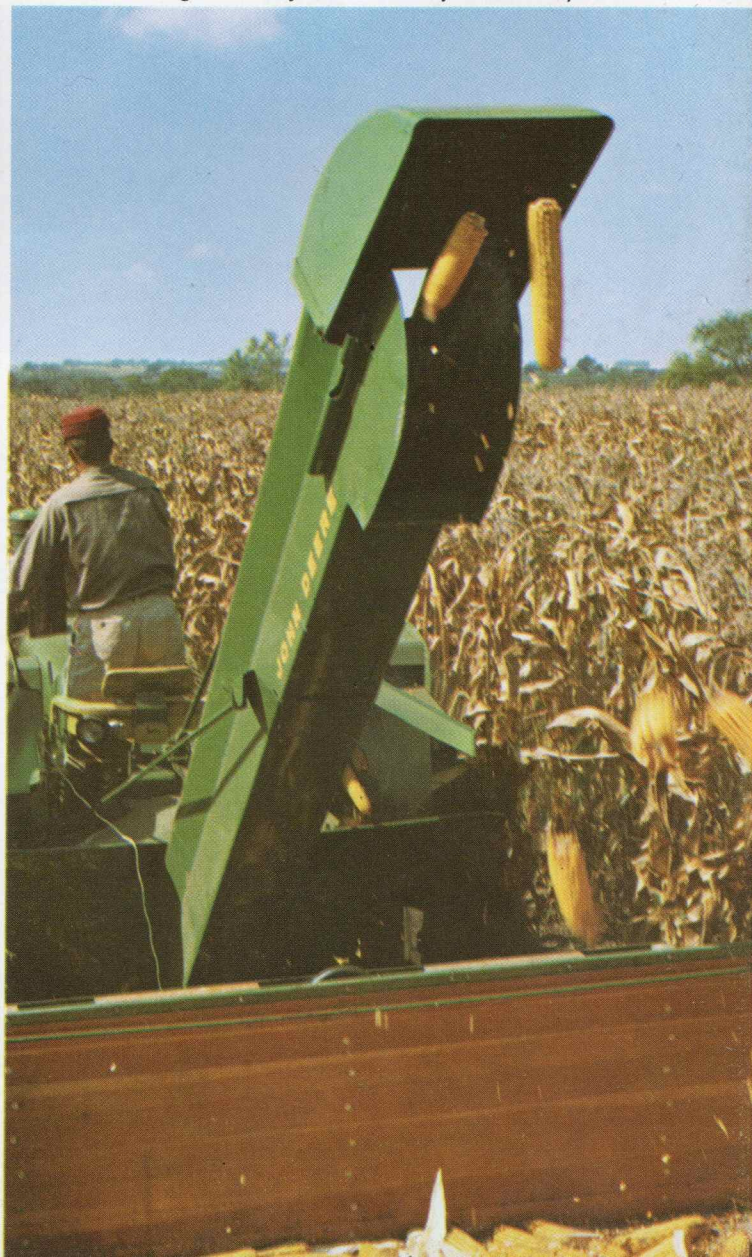
Load the wagon evenly with the adjustable deflector.
