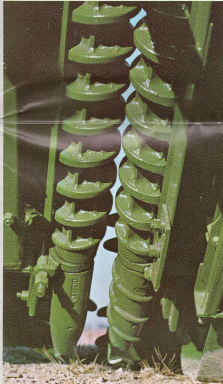
"Worm's-eye" view of snapping roll stripper bars.
