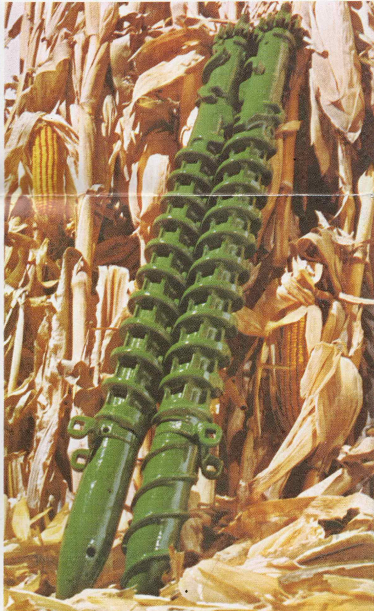
Spiral fluted snapping rolls cut shelling loss in half.
