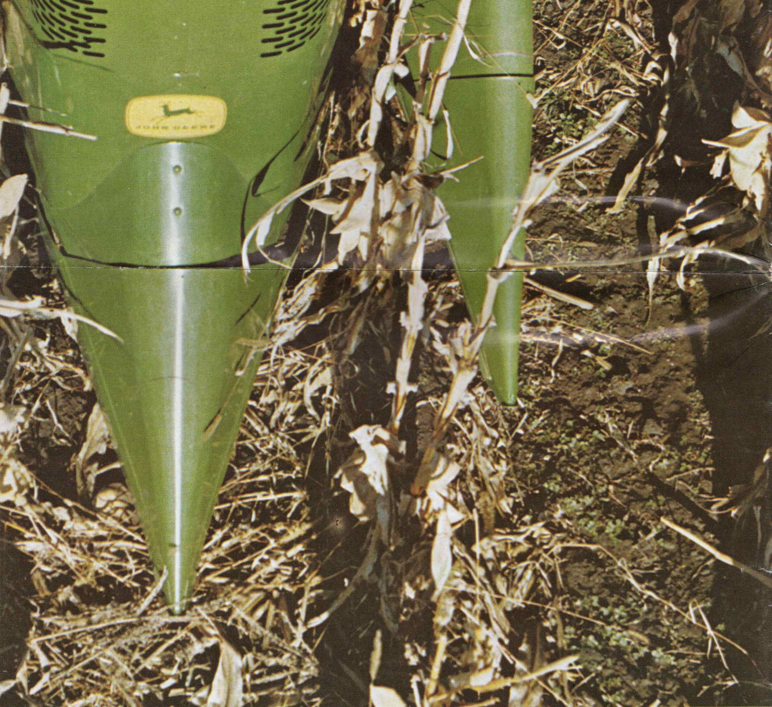
Slim, tapered "snouts" scoop up down stalks.
