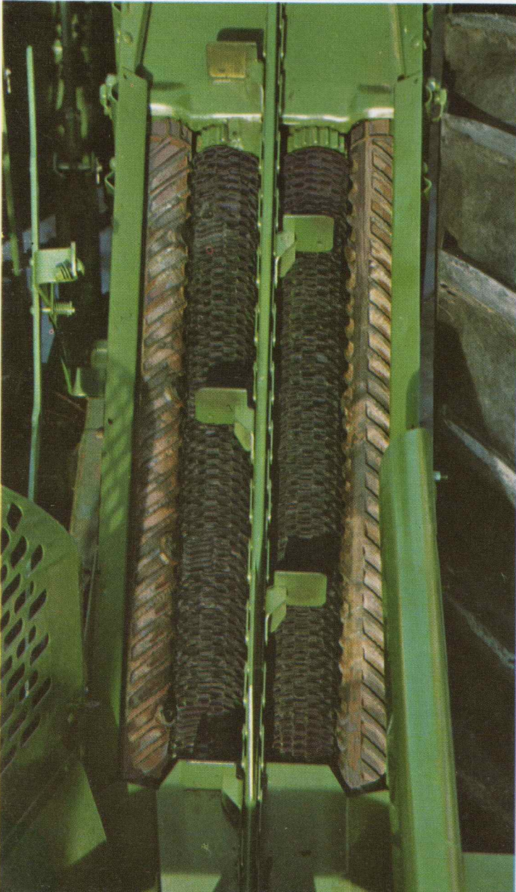
Husk clean with serrated rubber against steel spirals.
