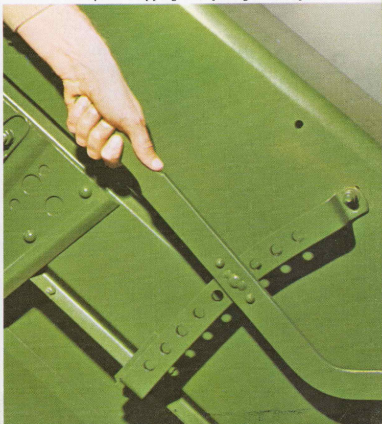
This lever adjusts snapping-roll spacing on the go.
