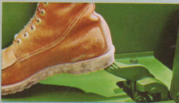
Depressing this differential-lock pedal can help keep you out of trouble and on the move in difficult conditions.
