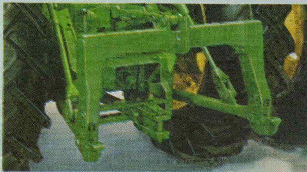
The Quik-Coupler Hitch is as sturdy as it looks; can be quickly adapted to Category 2 or 3 equipment.
