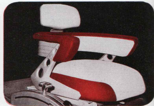
AIRLUXE SEAT: Unique oil/air suspension seat sets new standards in riding comfort. Fully padded armchair adjusts forward and back and hydraulic power adjusts up and down to match the operator's height and weight.
