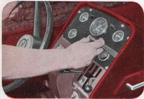
PANEL-MOUNTED CONTROLS: High-Low lever, gear change lever, throttle (an over-riding foot throttle is positioned near the right foot) Multi-Power switch and PTO clutch control are on the panel. Platform controls include hydraulic lift system, twin remote control valves, vertical seat adjustment lever and PTO selector.
