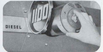
DRY ELEMENT AIR CLEANER: Most efficient, readily accessible, easy to service and clean. Air cleaner service indicator visually shows when element needs cleaning.
