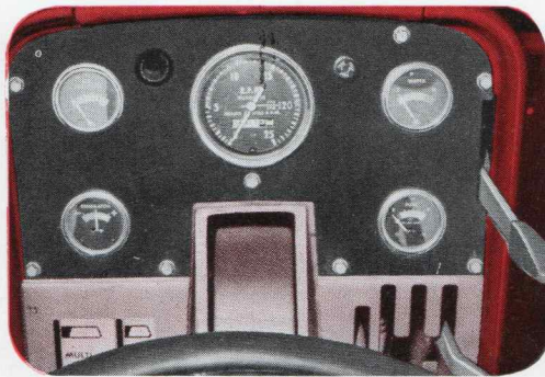
LUMINESCENT INSTRUMENTS: New type instrument lights eliminate bulk changing. Dial faces glow when the current is switched on. All instruments are enclosed in sealed, weatherproof cases. Panel includes tachometer with temperature gauge, fuel gauge, ammeter, oil pressure gauge.
