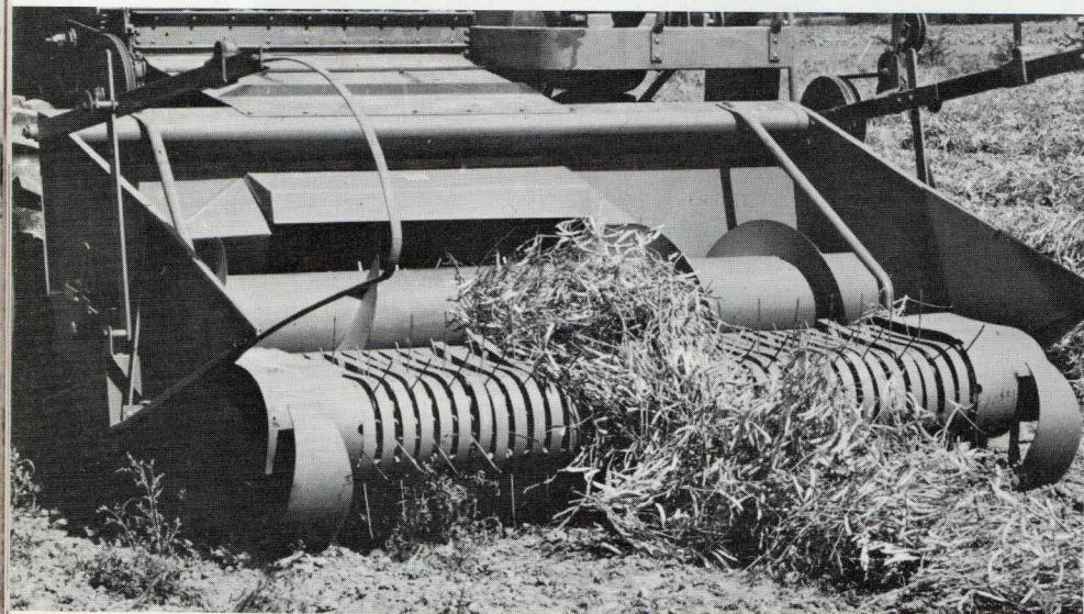
Windrow rotary type pick-up attachments in 8 and 10 ft. sizes are available for 10 and 13-ft. platforms. Gentle lifting action keeps shelling losses at a minimum . . . sweeps ground clean.
