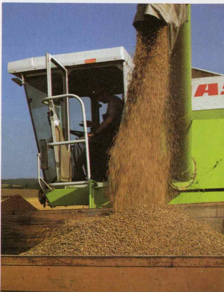
Quick grain tank discharging
