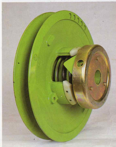
CLAAS automatic belt tensioning: reliability
