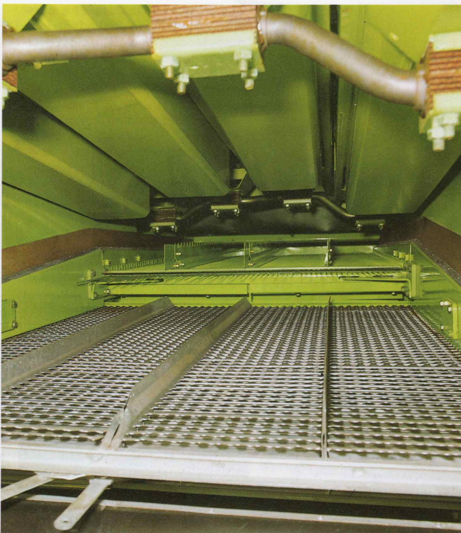
Large cleaning area, adjustable frogmouth sieves, continuous throughput monitoring
