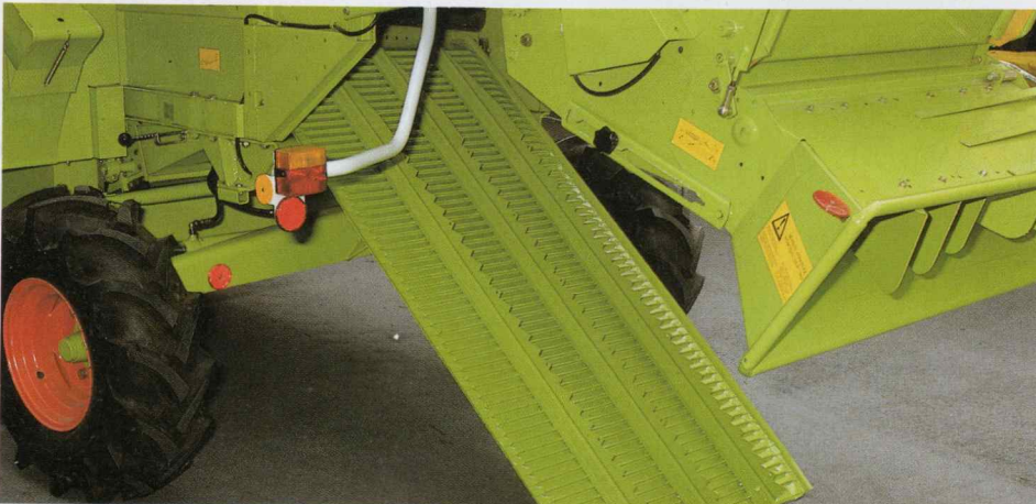
Easy cleaning facility for the preparation floor
