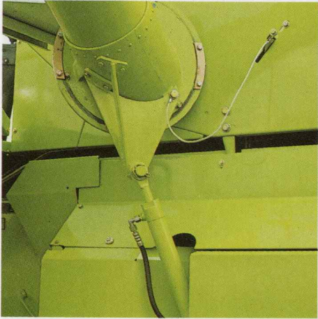
Grain tank auger: no losses here
