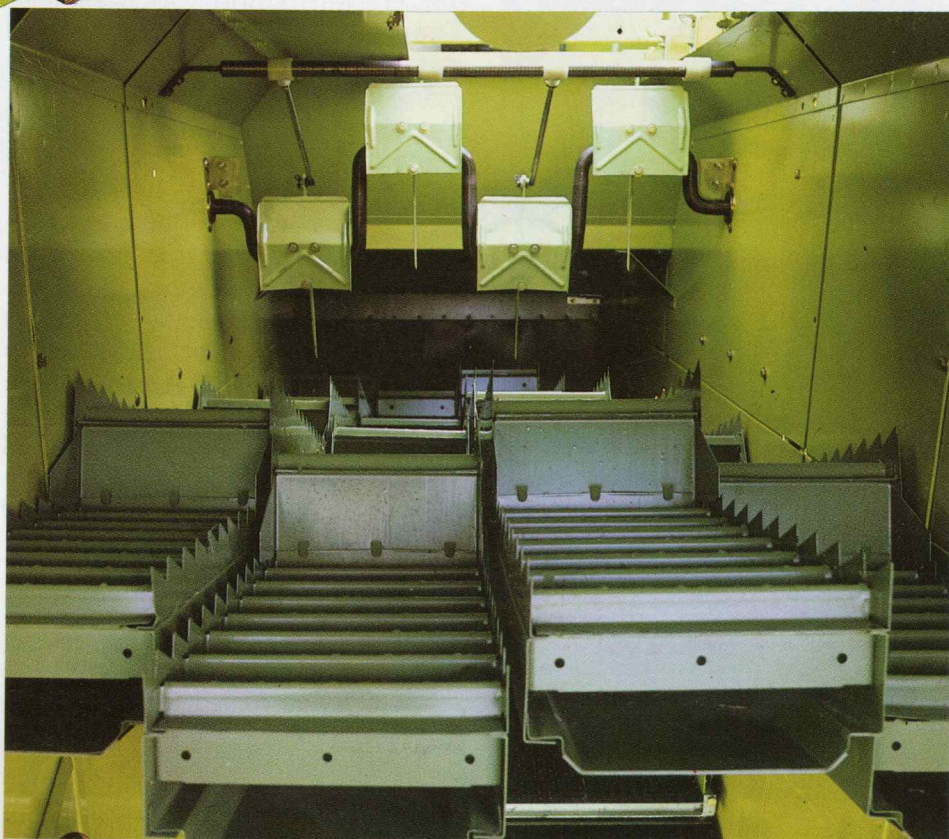
CLAAS separation system on the DOMINATOR 58
