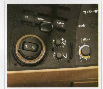
New electronic hitch control provides preselection which makes operation both quick and convenient.
