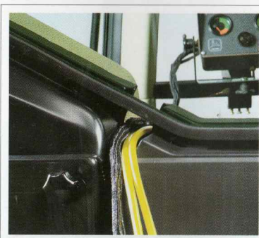
The tractor cab stays closed and sealed when you use this optional routing system for implement monitor cables.
