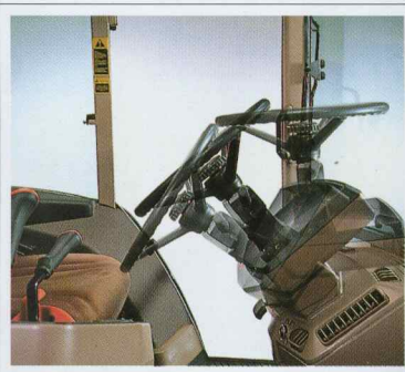
When you adjust the tilting and telescoping steering wheel, the instrument pod tilts with it. You always have a perfect view of the gauges.
