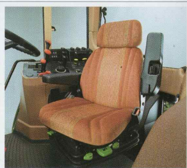
The Air Comfort Seat features adjustments for size, backrest, horizontal suspension and 200° of swivel control. The seat automatically compensates for your weight.
