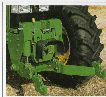
An integrated front PTO is available to help increase your productivity. A range of front hitches is available as allied equipment (depending on country).
