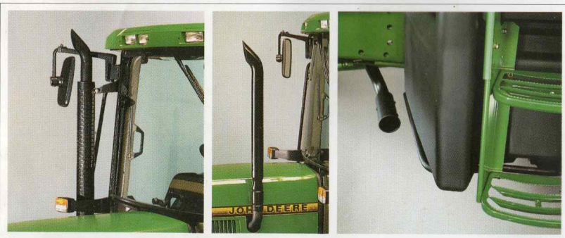
Three different exhaust stack options are available: cornerpost, vertical and horizontal (horizontal not for 6600 and 6800 tractors).*
