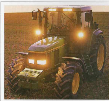
Four roofline and two beltline worklights (opt.) brighten up fieldwork at night. Up to 3 rear worklights complement the all-round illumination.
