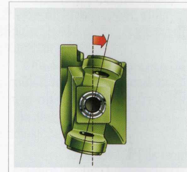
12-degree caster angle gives John Deere tight 4-wheel drive turning.
