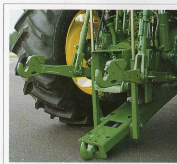
The new push-back pick-up hitch gives you an excellent view of the hook for easy coupling.
