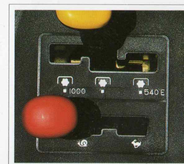
A creeper, available on all transmission versions, gives forward speeds as low as 60 m/h – that's just 1 metre per minute!
