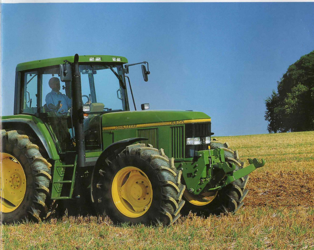
Heavy-duty front axle features integrated balanced steering and caster angle for outstanding manoeuvrability.
