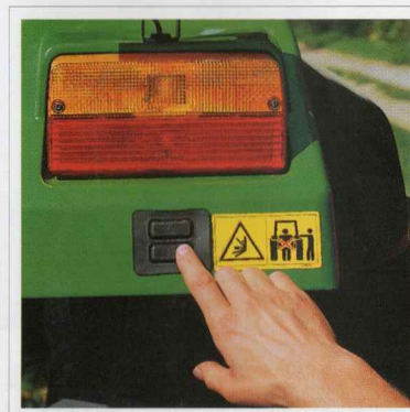
Fender-mounted remote control switches make 3-point hitch implement hookup easier.
