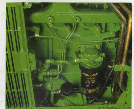
The fuel filter is behind the left hand engine compartment door.
