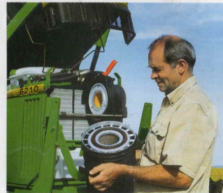
The air cleaner can be inspected by simply raising the hood.
