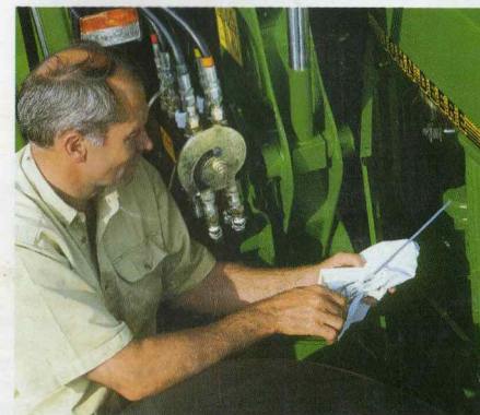
Engine oil levels and filter can be checked or changed by opening the right hand engine compartment door.
