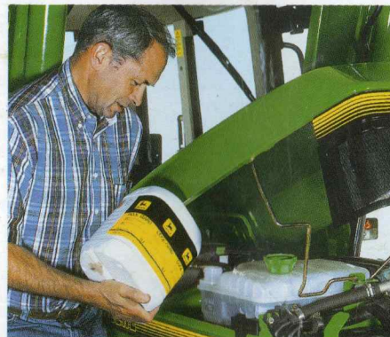
The coolant tank is easily reached with the hood propped open.
