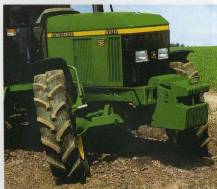
Tight turning 4WD provides extra traction in slick conditions. Caster action tilts and tucks the tyres under the frame for tight turns.
