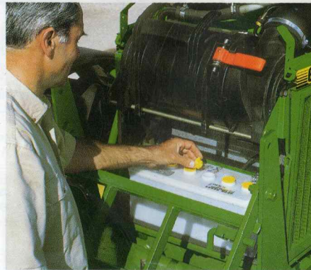
Just raise and prop the hood and remove the front panel for access to the battery.
