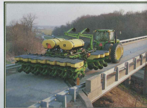
The double-duty 16/31-row 1780 (left) gives you 16 rows on 30-inch spacing and 31 rows on 15 inches.
