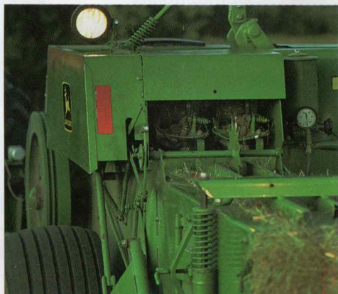
Auxiliary lights (optional) light up the pickup, knotter, and twine box for nighttime baling.
