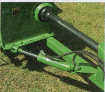
Hydraulic tongue positioning (optional) lets you switch from transport to field position from the tractor.
