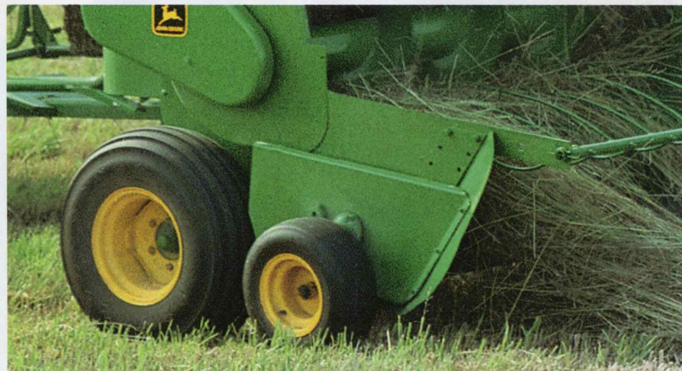
Pickup gauge wheels (optional) allow the pickup to float over uneven terrain, such as irrigated or rough fields, with less scalping. These high-flotation tires (16x6.50-8) provide smooth operation, and are adjustable for accurate ground gauging.
