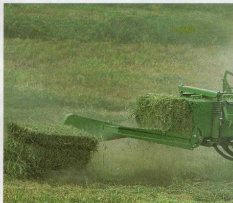
The optional side-drop chute places bales on their side to keep twine, or wire, off the ground. It's reversible, allowing either right- or left-side drops.
