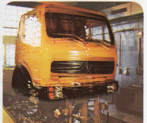
Magnetic tapes with load data from very bad surfaces and country roads control hydraulically driven simulators.
