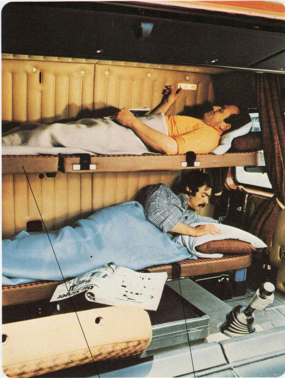
The two well-padded bunks in the long cab, each 60 cm wide, for rest and relaxation.
