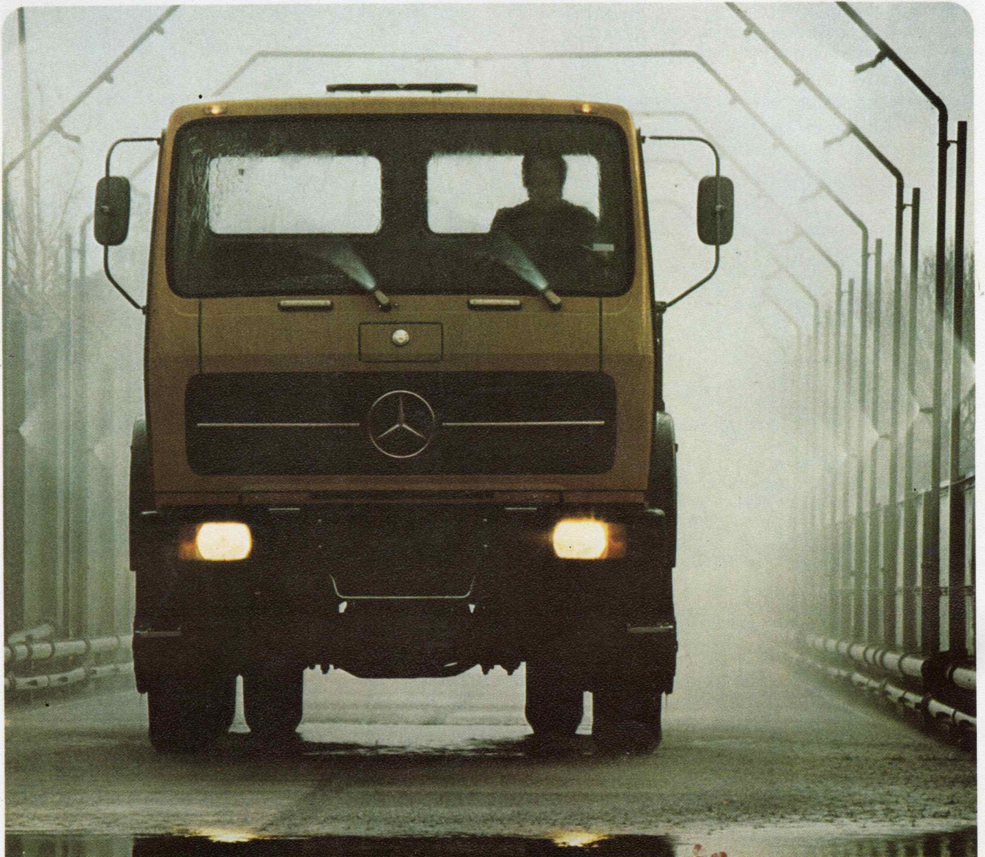
Artificial monsoon rain: about 70 litres of water per second pour down onto the track in this test carried out to detect whether the flaps, air inlets, doors or windows are leaking.
