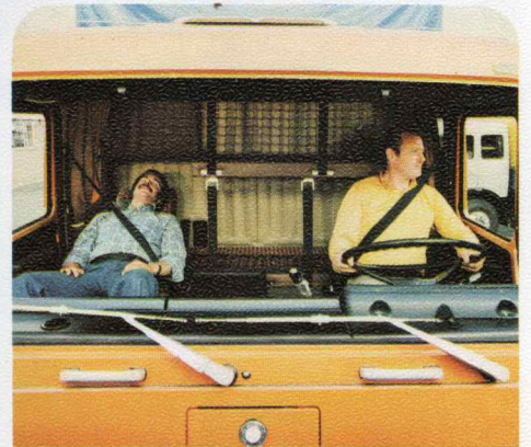
The upper bunk is divided, and the part behind the co-driver's seat can be folded back so that this seat (with armrest and head restraint) can be tilted a long way back - for relaxation during the journey.
