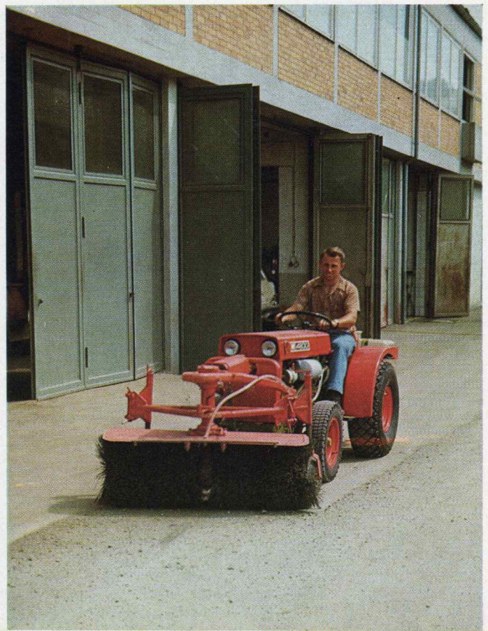
The front-mounted sweeper — brush width 120 cms. (48 ins.), 45 cm (18 in.) dia. — has 2 brush speeds (dust and snow) and can be swiveled to either side. Also available 100 ltr. (22 gals) capacity water tank, pump and sprinkler.
