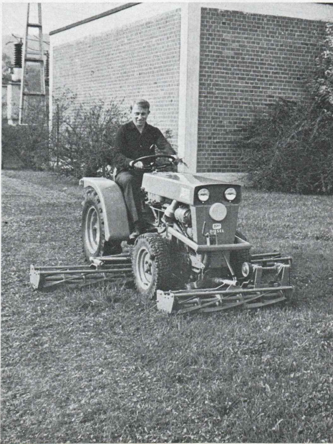
This 3-sectional reel mower has one reel mounted at the front and one mounted at either side. Working width: 230 cms. (90 ins.). The side reels can be raised alternately and held in the upright position. Mowing can also be carried out with the front reel alone.
