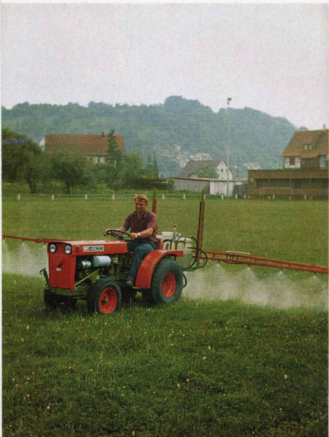
This area sprayer with low pressure pump and regulating device has an 8 mtrs. (26 feet) wide spray boom, 14 Teejet nozzles and 100 ltr. (22 gals.) capacity tank. The boom is adjustable in height from 70-130 cms. (28-51 ins.).
