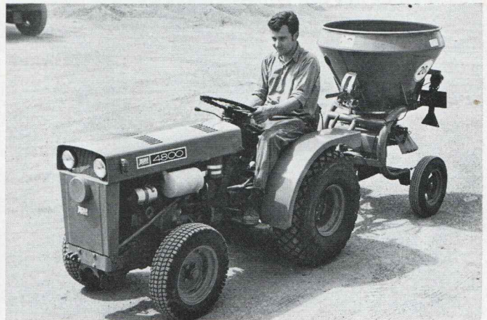
An all-weather hood protects the driver in bad weather. Sand, salt or fine gravel can be spread 2-8 mtrs. (6.5 - 26 feet) wide with this p. t. o. driven broadcaster with dosing device.
