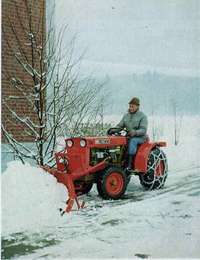
For quick clearance of fresh snow or light rubble we recommend this shock absorbing snow dozer 150 cm (59 in.) wide, which can be swiveled to either side and which is provided with steel or plastic edging. Operated from driver's seat.
