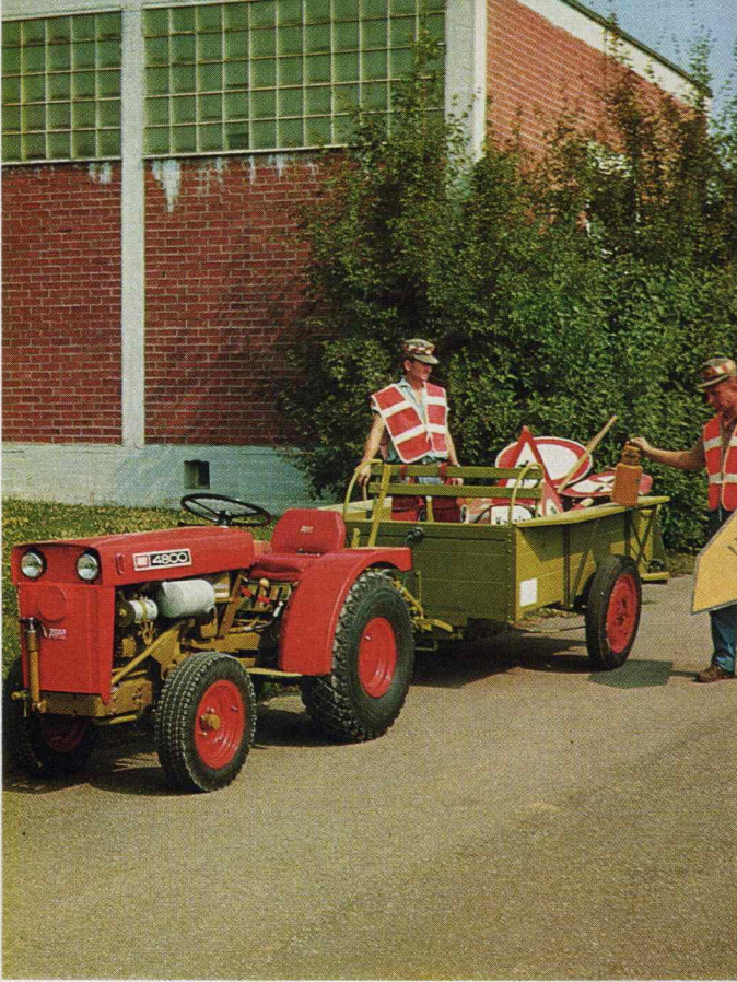
For transport purposes, 2-wheel or driven axle trailers with spring suspension and pneumatic tyres are available with 900 or 1400 kg. (approx. 18 or 28 cwts) carrying capacity. Max speed approx. 16.5 km/h (10 m. p. h.).
