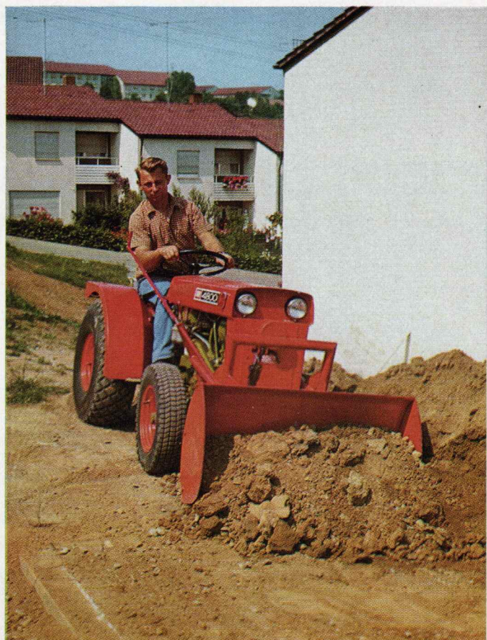
The oscillating, shock absorbing front-mounted earth dozer can be swiveled left or right from the driver's seat; is very robust and has a working width of 100 cms. (39 ins.). It is hydraulically raised and provided with side discs and steel blade edging.
