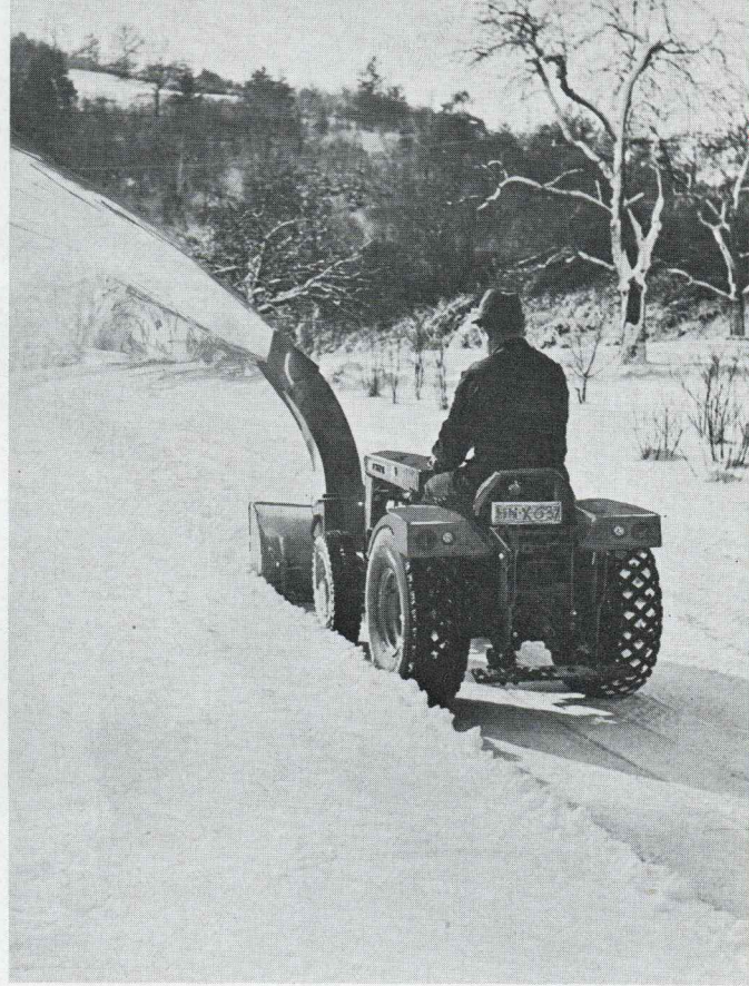
Larger amounts of snow can usually only be cleared by a snow thrower. The p. t. o. driven front-mounted snow thrower throws the snow to any side required and clears approx. 100 cms. (39 ins.) width.
