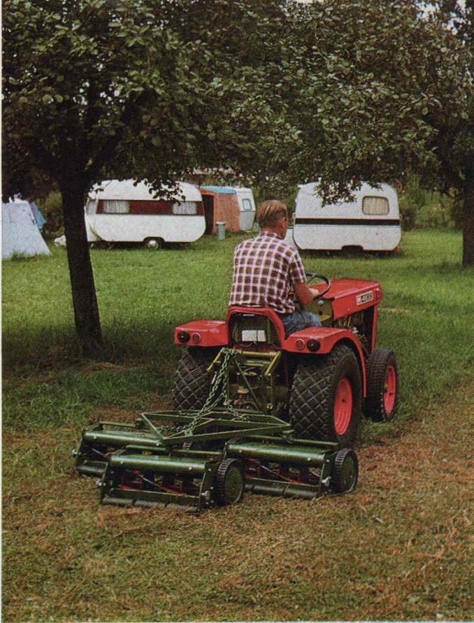
The 3-reel rear-mounted mower with hydraulic lift and 145 cm (57 in.) working width is ideal for mowing large areas. Mowing capacity at 6 km/h (3.7 m. p. h.) is 8500 sq. mtrs. The swing mounted reels adapt themselves well to unevenness of ground.
